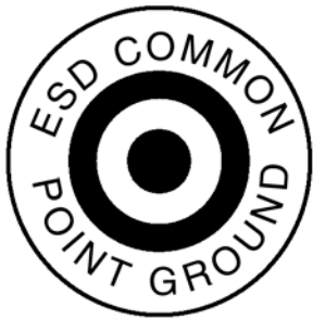
Figure 1: Common Point Ground Symbol
